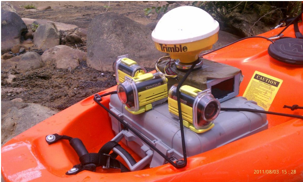
Figure 1 Streambank video mapping system
